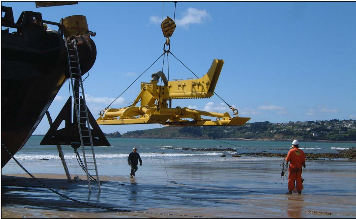
Figure 2-15. Example of Water Jet Trenching Device
